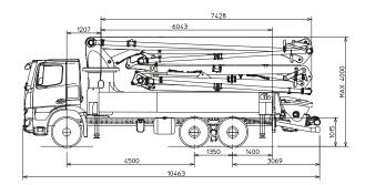
Dimensions varying according to truck assembly
